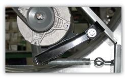
Belt drive models include a heavy duty spring belt tensioner to reduce bounce at startup and provide uniform loading to increase the life of the belt and maintain high efficiency.
