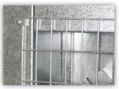
Removable 12 Gauge 1" x 2" wire mesh guards are hot dip galvanized after welding. The guard is attached to the housing with poly guard clips to reduce noise and vibration.
